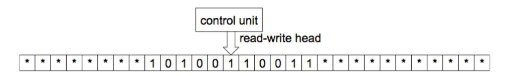
The computation of a Turing machine is controlled by a *transition function*:
