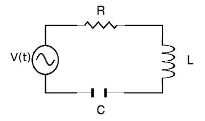
Fig. 30: An *LRC* circuit
