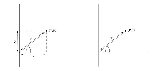
**Fig. 24:** The Cartesian and polar coordinates  $(r, \theta)$  of a point
