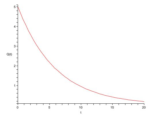
Fig. 27: A discharging capacitor
