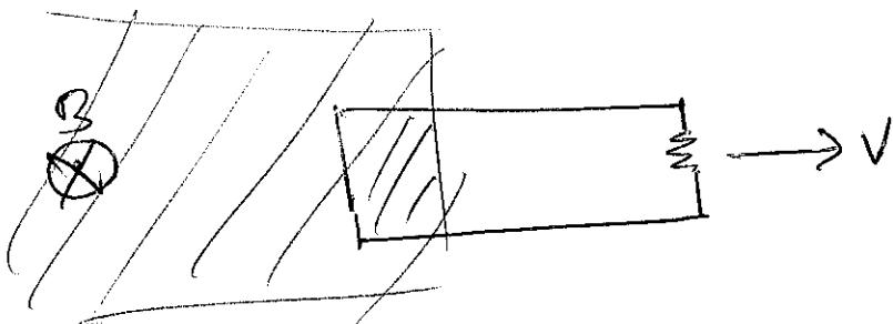
Flux decreases, magnetic force causes charges to move, drives current. (EMF generated)
