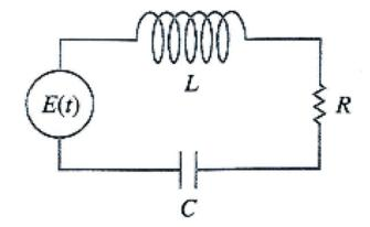
According to **Kirchhoff's second law**, the impressed voltage E(t) must equal to the sum of the voltage drops in the loop.
